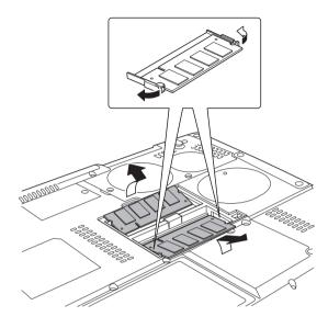
Figure 8-5 Removing the memory module
